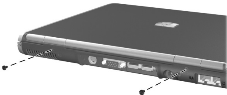
Removing the Display Assembly Screws
